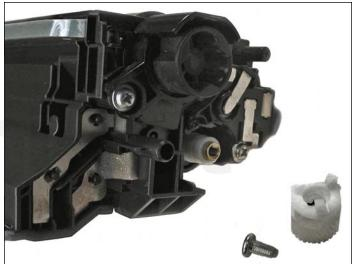
25. Using a Phillips screwdriver, remove the screw from the developer roller drive gear, and remove the gear.
