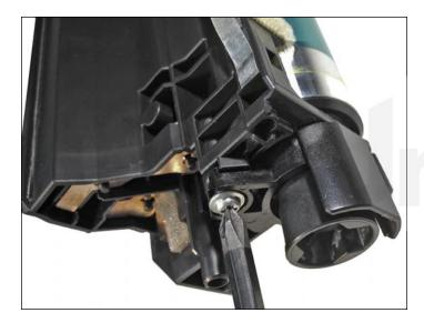
**DISASSEMBLING THE DRUM UNIT**28. Remove the screw from the OPC drive gear support plate shown.
