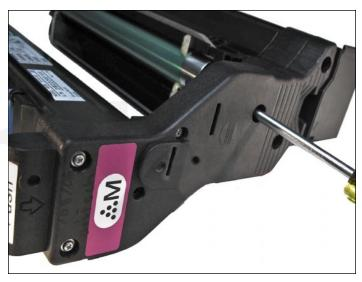
53. Secure the outer end cap with the seven screws.
