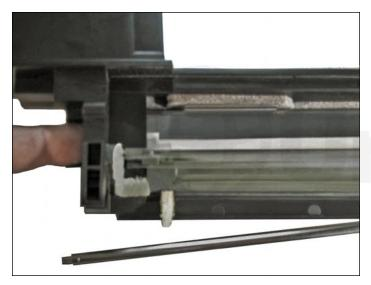
37. Once the corona wire is aligned with the cartridge, push in with your finger until it is back into its original place.
