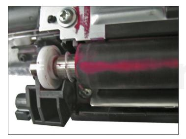
16. Take special note of the center position of developer roller washer, located at the ends of the developer roller axles. Remembr this when installing the developer roller as per OEM.
