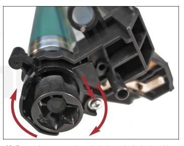
40. Rotate the support plate clockwise to its locked position.
