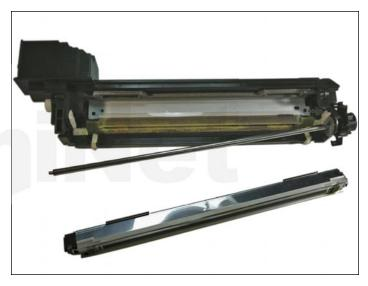
33. Remove the corona wire by sliding it in towards the opening on the gear train side (A), then pulling it out (B).
