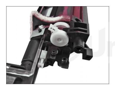
14. Remove the **capped** developer roller support bearing on the non-contact end cap side.
