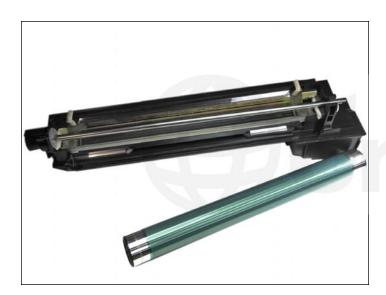
32. Wipe the removed OPC with drum cleaning solution. Cover and set the drum aside.
