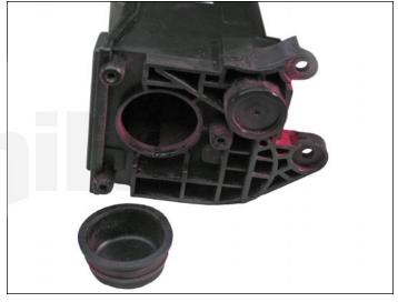
3. Locate the toner hopper fill plug, and remove it by prying it off, using a small flathead screwdriver.
