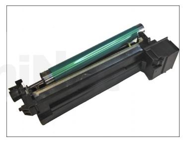
38. We are now ready to install the OPC drum. Before installing, make sure the drum gears are facing the corect position. Slide into place via the axle.
