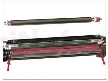
17. Remove the developer roller as shown.
