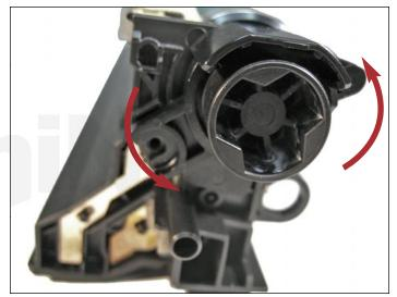
29. With the screw removed, turn the support plate counter-clockwise until it comes to a stop. This will unlock the plate and allow you to remove it completely.
