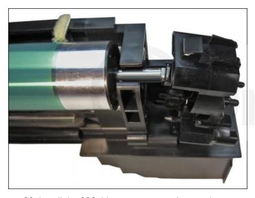
39. Install the OPC drive gear support plate as shown.
