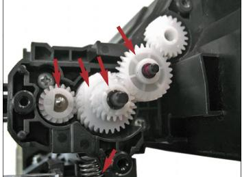
45. With the two haves assembled, proceed to install the gear train and the appropriate springs.
