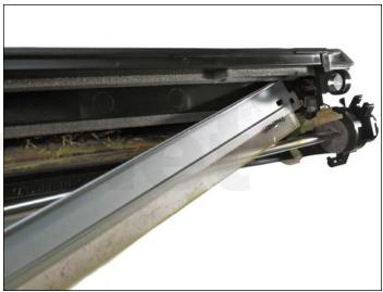
34. Remove the two wiper blade screws, and remove the wiper blade.
