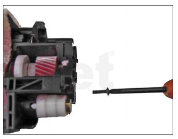
5. The contact end cap will have a smaller screw that will also need to be removed.
