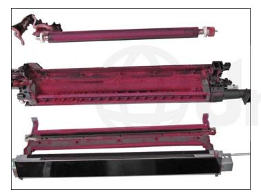
20. Clean the disassembled developer section with a vacuum.
